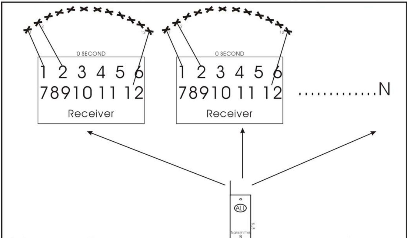
6, Cancel all the frequencies previously programmed into the receiver first. Then get one transmitter B to be programmed to many(N) receivers.
