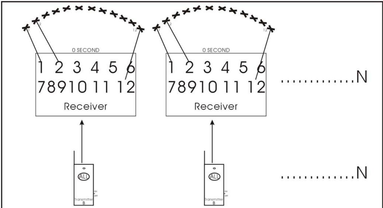
5, Cancel all the frequencies previously programmed into the receiver first. Then different transmitter B will be programmed to different receivers separately.
